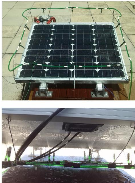
Figure 10. Front and back surfaces of the PV panel with a specific water nozzle system integrated
