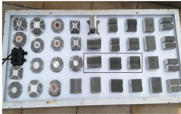
Figure 3. The back side of the passively cooled panel has heat sinks with different geometries
