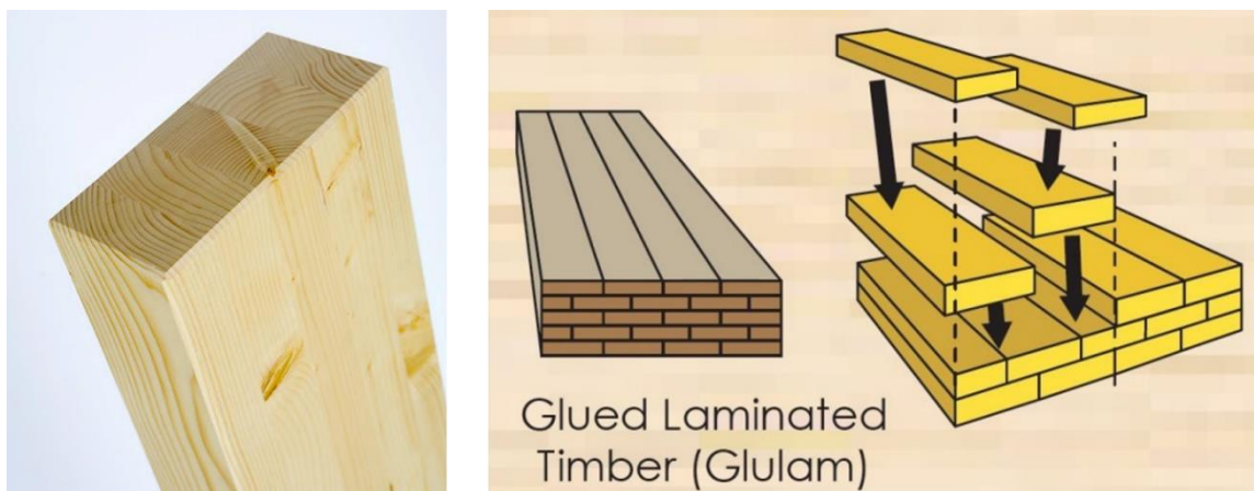
Figure 11. GLULAM and positioning of timbers used in GLULAM construction (URL-7).
